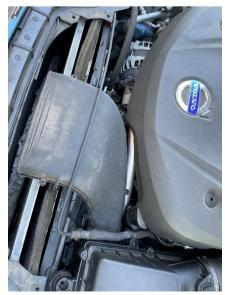
Undo the small coolant line from it's fastening points and place it on top of the intake duct, and unclip the line also from the side of the air filter housing.
