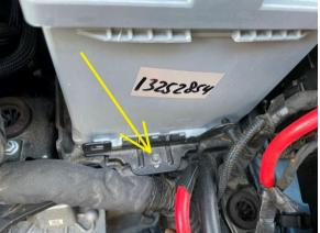
Remove battery and battery tray.
