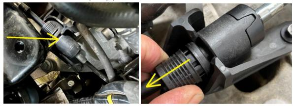
Pull back the secure ring (see picture) and undo the shift cable from the cable bracket.
