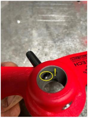
Put the M66-Shift Short Shifter on the shift shaft and press the secure pin all the way in the shifter arm with groove joint pliers. (Dutch: Waterpomptang)
