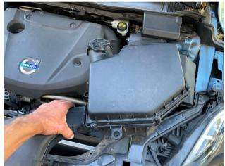
Pull the air filter housing up (from it's rubber mounts), and remove it. Remove the battery protection plate and unscrew the cable connections from the 12 Volt distribution block which are shown in a yellow circle.
