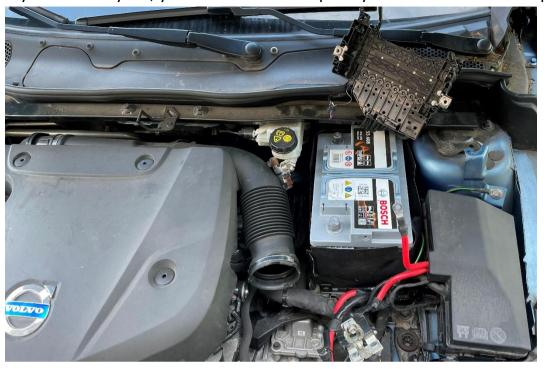
Remove battery insulation, and unscrew the battery secure bracket.
