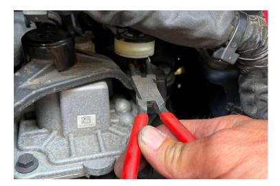
Underneath the battery tray you will find the shift cable bracket.
